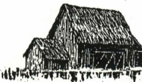
PIONEER BARN Featured wooden hinges, open slit-window ventilation, steep thatched roof and attached sheds.
